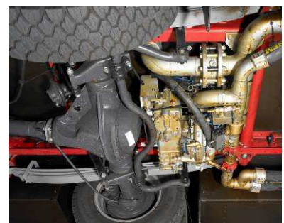
Built in as underfloor pump: More space for equipment or a portable pump
